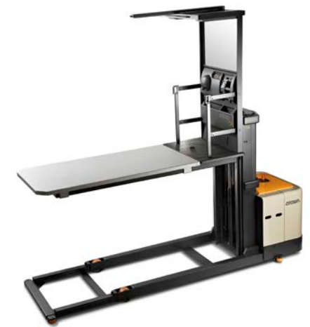
SP 3570F Series Straddle Load Capacity: 3000 lbs Lift Height: 210 to 366 in
