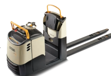
GPC 3000 Series Low Level Order Picker Load Capacity: 6000 lbs Forks: Available only in double length Platform Lift Available
